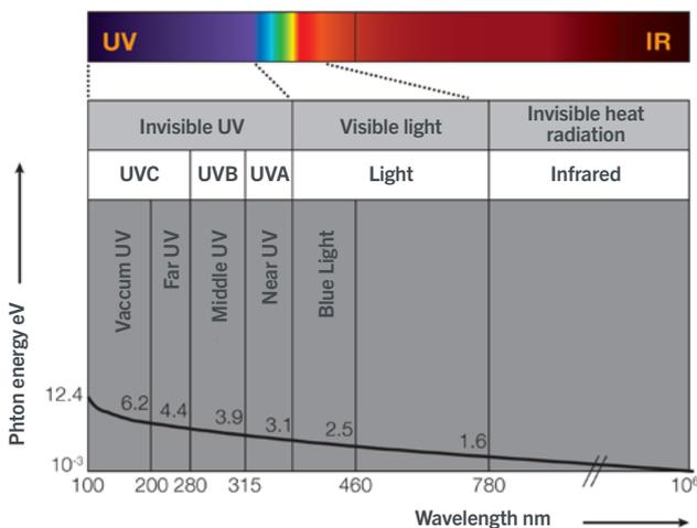
FIG. 1 | Radiation as a function of increasing photon energy.
