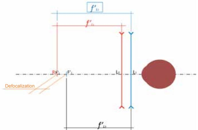
FIG. 6 | Variation in the correction of myopia with the vertex distance (d). The lens movement from L0 to L1 causes defocusing. The focal length of the corrective lens becomes  $f'L1 > f'L0$ . To compensate myopia, the power should be decreased if the lens is closer to the eye.
